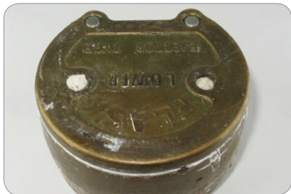
6) With the wax denture fixed, connect the flask wall and inject plaster completely. Cover to remove the air inside.
