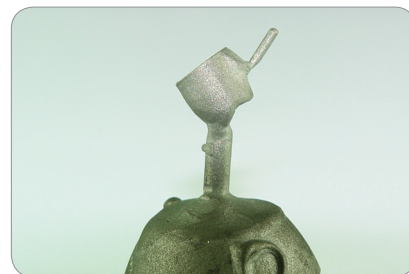
3) Body completed via centrifugal casting machine
