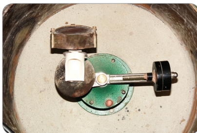
2) Centrifugal casting machine used commonly for casting
