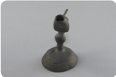
3) PFM model with completed casting
