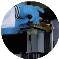
② Removal of output board
